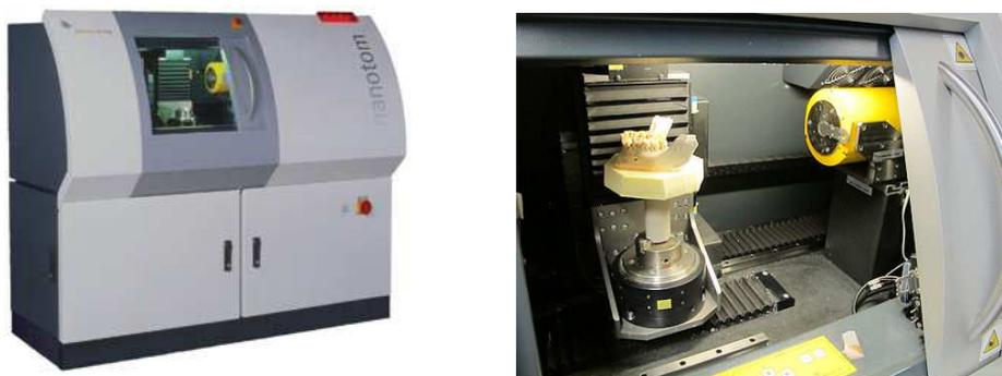
Image 4. The Phoenix nanotom (left) and the mandible placed in the CT scanner (right)
