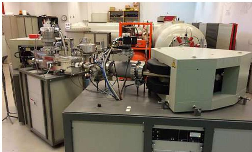
*Image 8. Particle Accelerator for Radio Carbon dating at the Groningen University*
